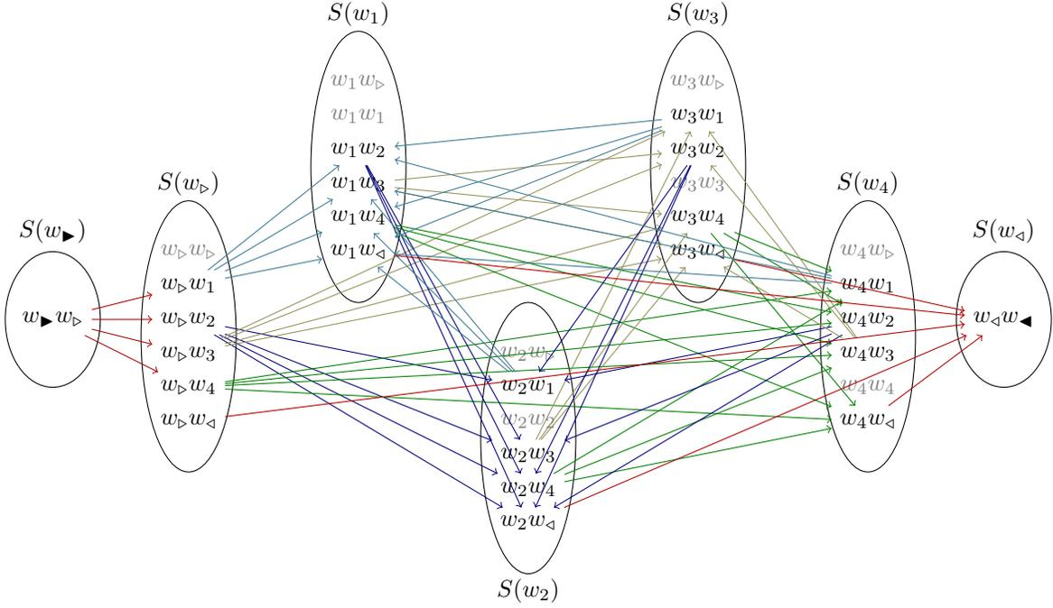
Figure 2. A graph showing the legal transitions between states, when the word-ordering problem is expressed similar to a GA-TSP. Each edge  $\langle w_a, w_b \rangle \rightarrow \langle w_c, w_d \rangle$  has cost  $-\log(P(w_c|w_a w_b))$ . The nodes are grouped into districts (words). Nodes for invalid states are greyed out.
